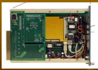
PC104plus PC board computer PCM-9370's Crusoe TM5400, Memory, Flash Disk, Ethernet, USB, ...
