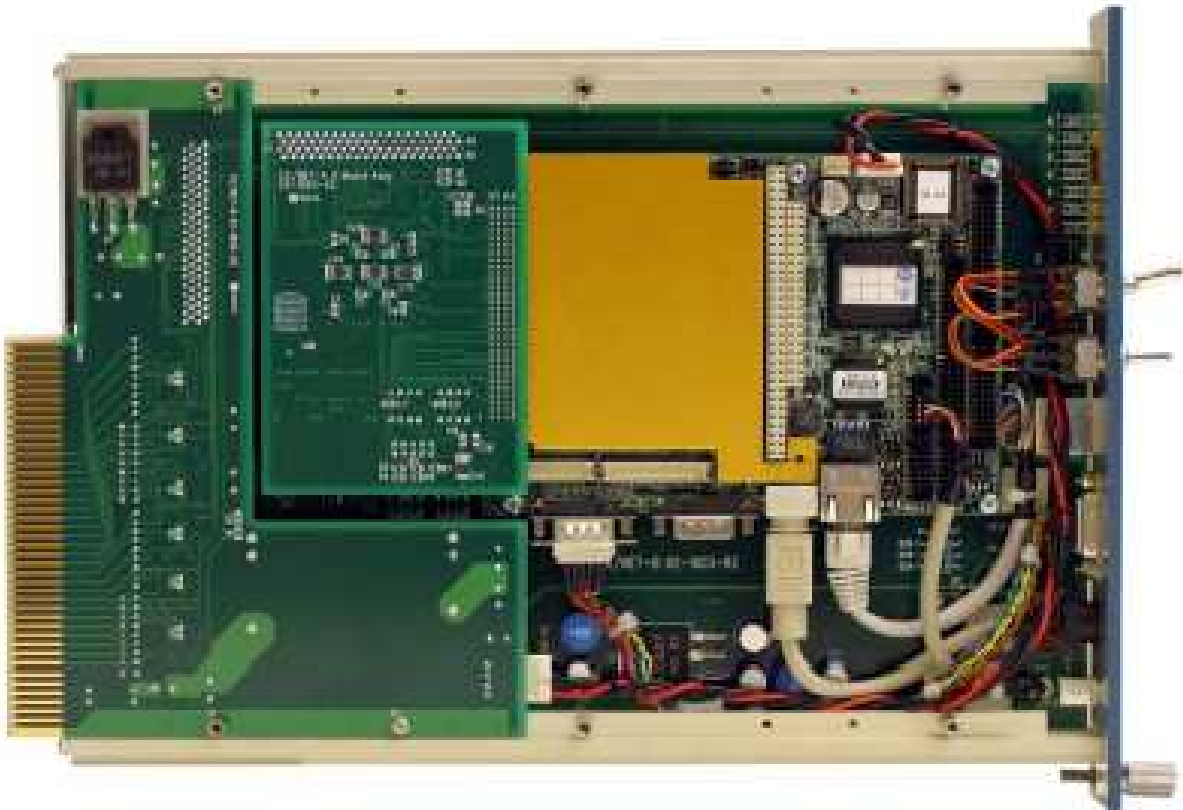
Figure 2.1: pipeline CAMAC controller
