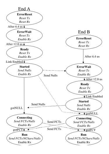
Figure 7-5 Example: Typical Initialisation Sequence
