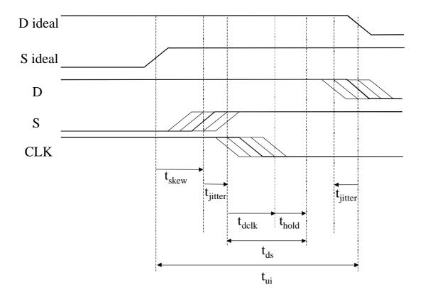
Figure 5-3 Skew and Jitter
