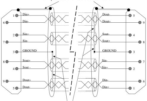
Low impedance bond from outer braid to connector shell
