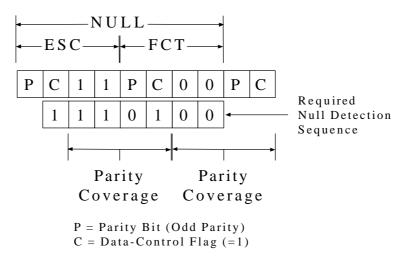
**Figure 7-3 NULL Detection Sequence**
