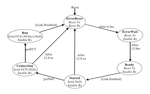
Figure 7-4 Basic State Diagram for SpaceWire Link Interface
