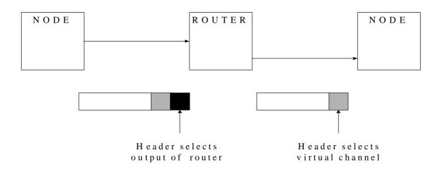
Figure 9-3 Header Deletion
