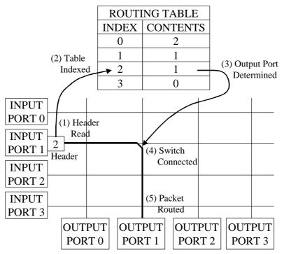
Figure 9-6 Example: Indirect Output Port Addressing via a Routing table.
