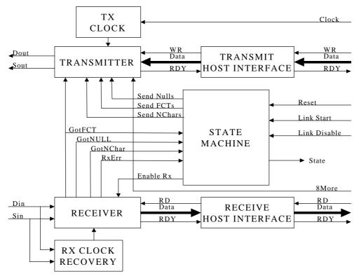
Figure 7-1 Example SpaceWire Link Interface Block Diagram
