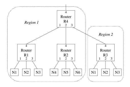
Figure 9-9 Example SpaceWire Network with Local Logical Address Regions
