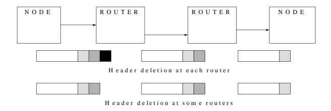
Figure 9-4 Header Deletion Across Multiple Switches
