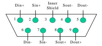
Figure 4-2 SpaceWire Connector Pin-Out
