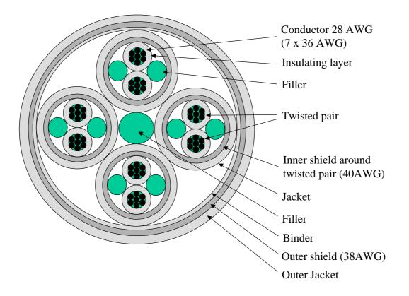
Figure 4-1 SpaceWire Cable Construction
