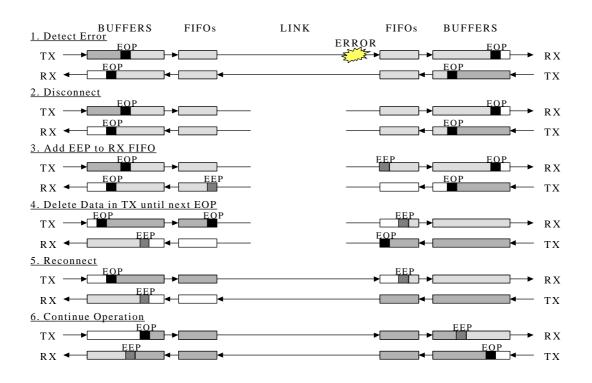
Figure 10-1 Link Interface Error Detection and Recovery Operation
