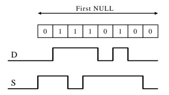
Figure 6-4 Data and Strobe Signals on Link Start
