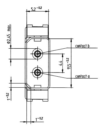
Figure B.1 —HS-SE free connector front view
