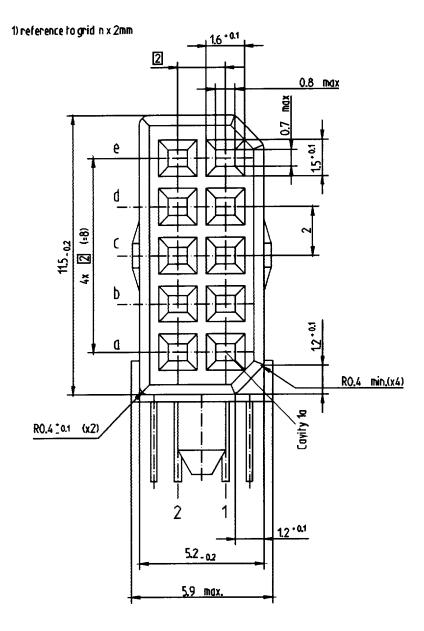
Figure A.1 — DS-DE fixed connector front view
