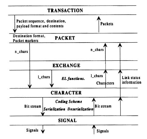
Figure 4-3 — Protocol stack diagram showing interaction of layers
