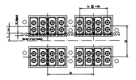
Figure Q.1—HS-SE multiway housing
