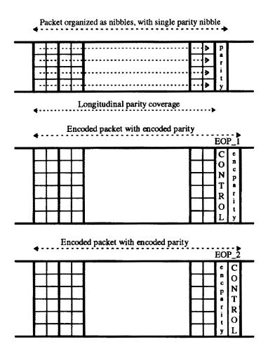
Figure 6-7 — TS-FO packet encoding
