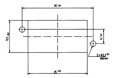
Figure Q.2—HS-SE (multiway) front panel cut out
