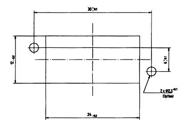
Figure N.2—DS-DE (multiway) front panel cut-out
