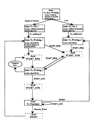
Figure 7-7 — Transmitter state machine controller—start-up
