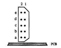
Figure 5-7 — DS-DE fixed connector external view
