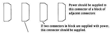
If three connectors in block are supplied with power this connector should be supplied
