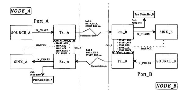
Figure 7-6 — Exchange level interconnection between two nodes
