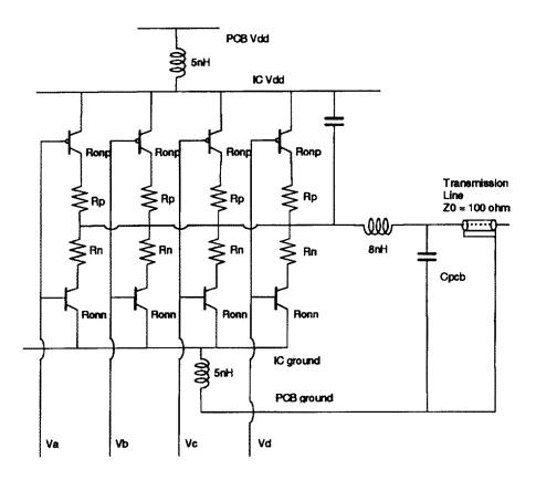
Figure J.1—S-SE pad equivalent circuit
