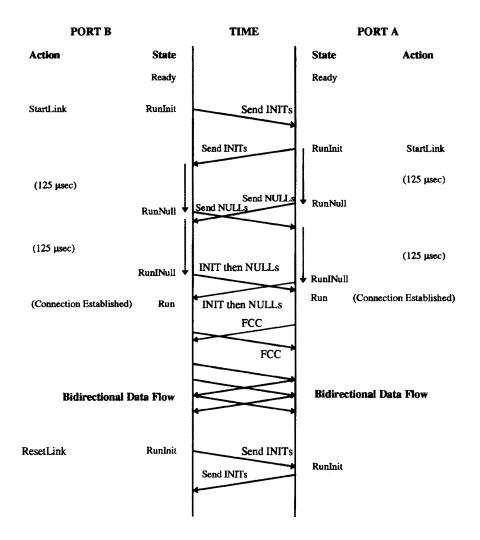
Figure 6-6 — TS link start-up and reset
