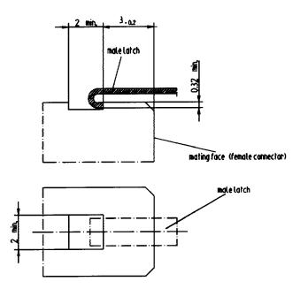
Figure B.5 —HS-SE connector link
