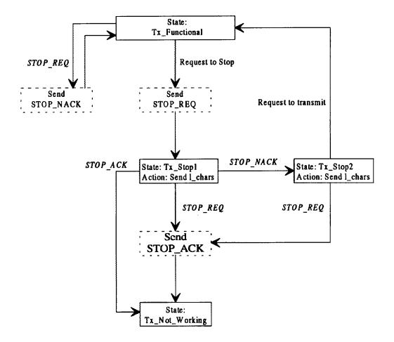
Figure 7-9 — Transmitter state machine controller—shutdown
