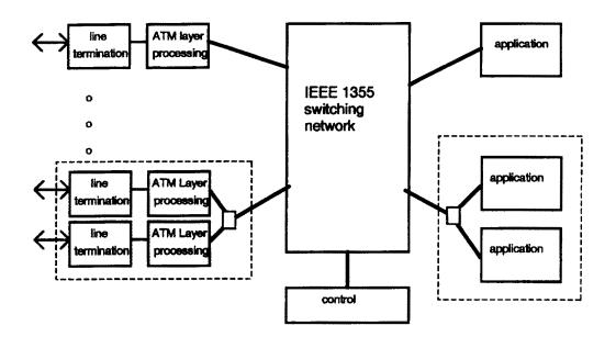
Figure F.6 — Mapping reference model
