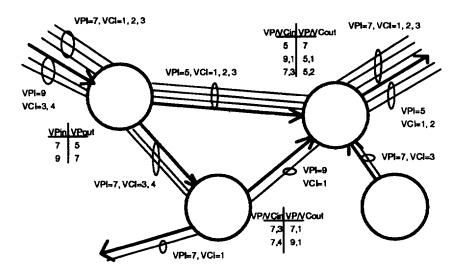
Figure F.4 — Example of virtual path and virtual channel switching
