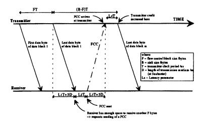
Figure H.1—Theoretical maximum transmission length calculation
