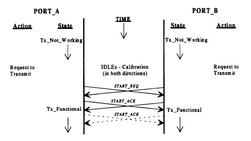
Figure 7-12 — Exchange for bidirectional start-up
