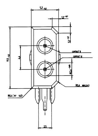
Figure B.3 —HS-SE fixed connector front view
