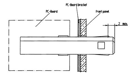
Figure A.3 — DS-DE fixed connector top view
