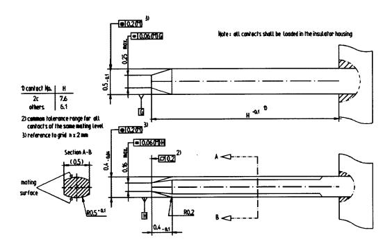
Figure A.7 — DS-DE free connector contact
