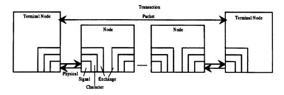
Figure 4-1 — Protocol stack between nodes
