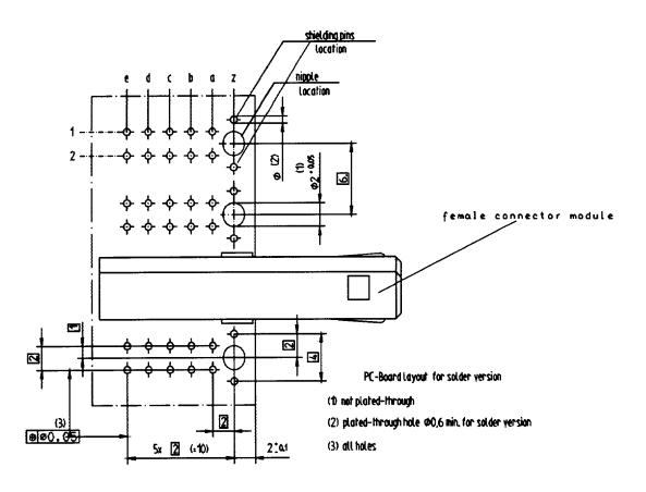
Figure L.1—DS-DE fixed connector PCB layout
