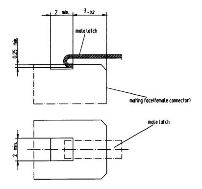
Figure A.4 — DS-DE connector latch
