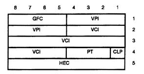
Figure F.5 — ATM cell header
