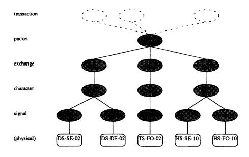
Figure 4-4 — Defined implementations of physical and logical layers
