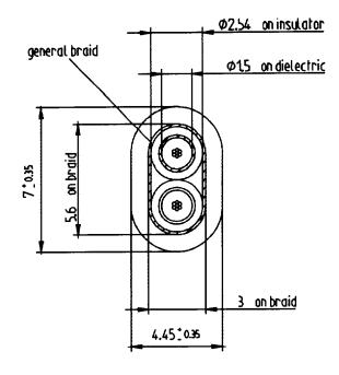
Figure P.1—Recommended HS-SE link shielded cable cross section
