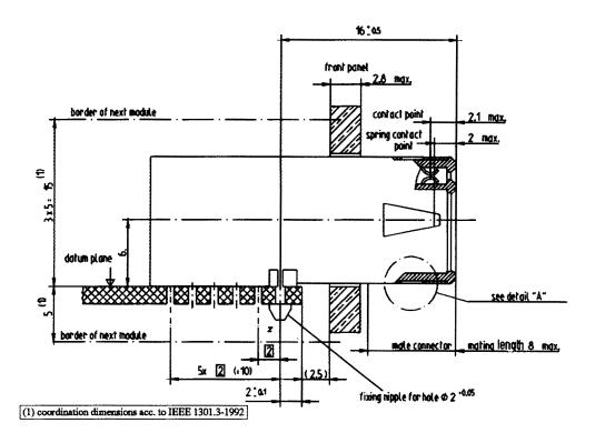
Figure A.2 — DS-DE fixed connector side view
