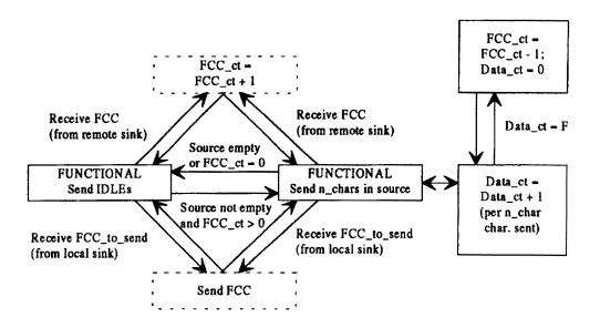
Figure 7-8 — Transmitter state machine controller—functional
