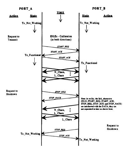
Figure 7-11 — Exchange for start-up, functional and shutdown
