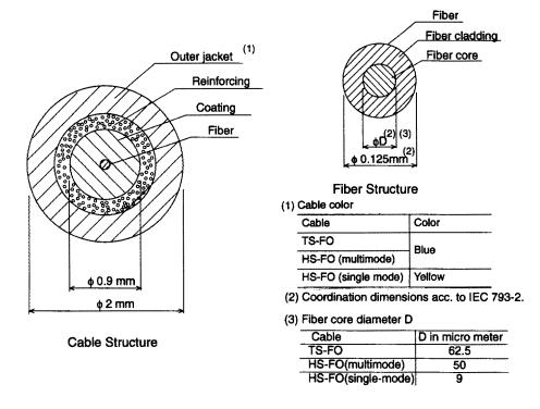
Figure S.1—Example of TS/HS-FO fiber cable structure
