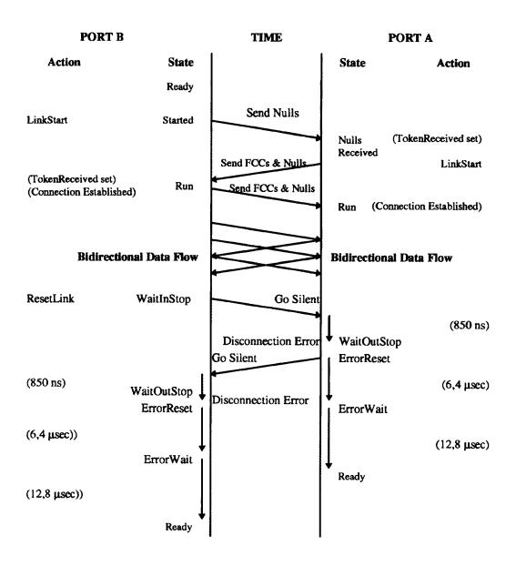
Figure 5-12 — DS link start-up and reset
