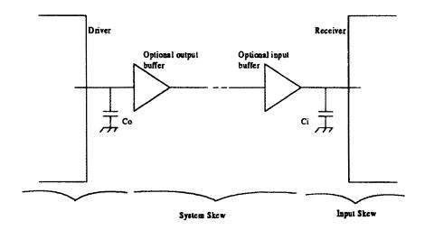
Figure 5-2 — DS-SE timing reference model
