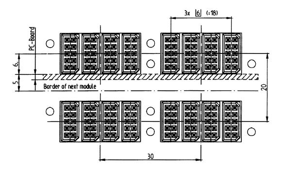
Figure N.1—DS-DE connector multiway housing
