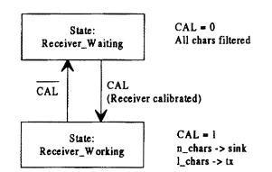
Figure 7-10 — Receiver state machine controller
