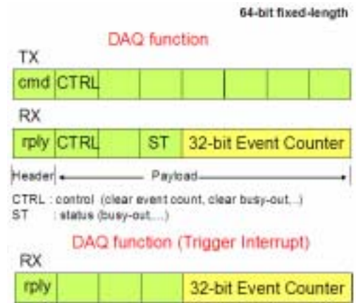
Fig. 5. Frame format of DAQ function
